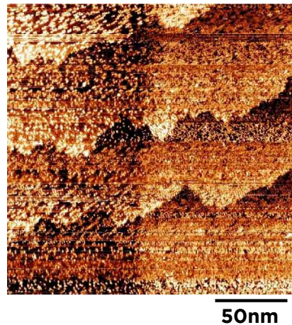
Figure 5.10: STM-based hydrogen desorption A close-up STM image of a desorption edge from a large-area rectangle pattern. The exposed silicon appears brighter due to the higher tunneling current obtained from the silicon surface states. Very sharp, well-defined desorption can be achieved with the STM technique.
